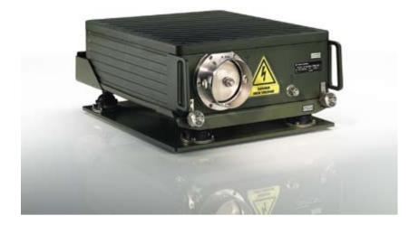
The HF Antenna Tuning Unit R&S®FK 3150 is part of the R&S®M3TR tactical transceiver family. It allows automatic matching of HF antennas, in particular of electrically short antennas, as are usually found in vehicular applications. The sturdy and water-proof casing of the R&S®FK 3150 is shock-and UV-resistant and thus ideal for mobile applications.
